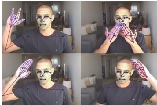
Fig. 3. Extraction of Keypoints from Video Sequences for Sign Language Recognition
